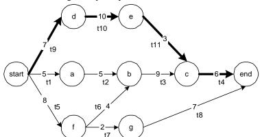
The chart above shows a project with many tasks and dependencies. At the start of the project three tasks (t1, t9, and t5) begin concurrently. Other tasks start as these tasks end. Notice that t6 and t7 cannot begin until t5 completes. Notice also that t3 cannot start until t2 and t6 both complete.
