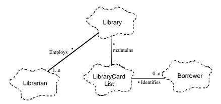
This diagram is called a class diagram. It is typical of those produced during object-oriented analysis. It is similar to an entity relationship diagram (ERD), except that it uses Booch symbols. It shows the classes in the model, and the static relationships between those classes.
