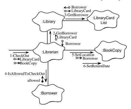
This diagram is called an object diagram. It shows the objects that we expect to participate in the behavior, and shows the messages and data that flow between those objects. Note that each message is numbered in the sequence that it occurs.
