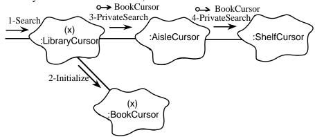
Here we see a client sending the Search message to object (x):LibraryCursor. The name of the object is 'x', but the parenthesis indicate that the name is local to this diagram, and not known to the rest of the design. It's kind of like a local variable. Object 'x' responds by sending itself the Initialize method, which is handled by the BookCursor base class. This method clears a set of counters in the BookCursor which keep track of statistics concerning the search.
